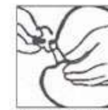
5. Pinch the upper end of the drain valve and open the plug to discharge
