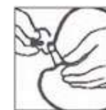
5. Pinch the upper end of the drain valve and open the plug to discharge
